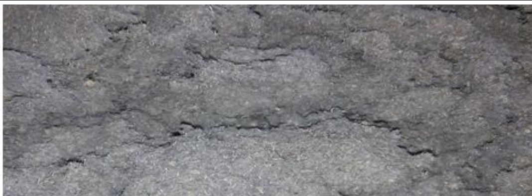
Plate IV: Chrome re-tanned powder (0.5mm size, using Arthur Thomas Wiley Laboratory mill model 4 USA) ready for compounding with HDPE.
