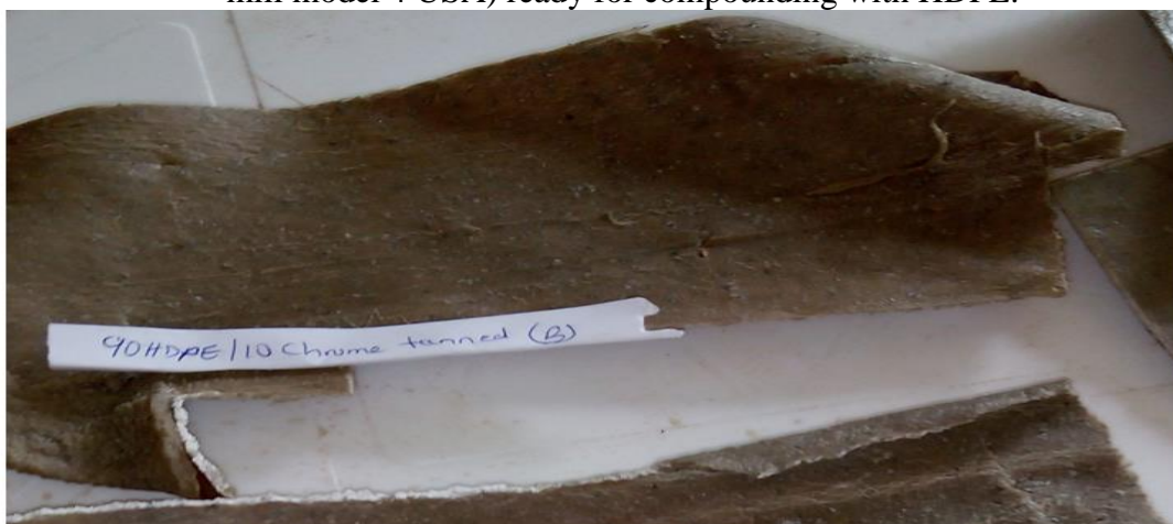
Plate V: Compounded sample with 0.5g trimethylquinoline (TMQ), 3.5g Mg(OH) 2 , 0.3g TiO 2 were used as additives
